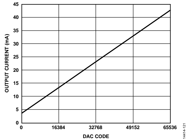
Figure 138. Gain Curve for ANA\_FULL\_SCALE\_CURRENT[9:0] = 1023 , DAC Offset = 3.8 mA
