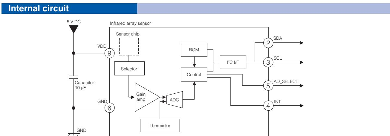
\* INT terminal ④ normally has same voltage as VDD. When interrupting, same as GND (0V)
