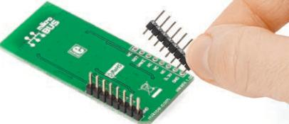
Turn the board upside down so that the bottom side is facing you upwards. Place shorter pins of the header into the appropriate soldering pads.
